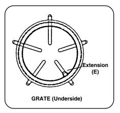
The five finger grates are porcelain enameled cast iron or steel and have an extension (E) that is longer (underneath) than the other four. This extension fits into the indentation (E) on the burner plate, which is directly across from the igniter (D).
